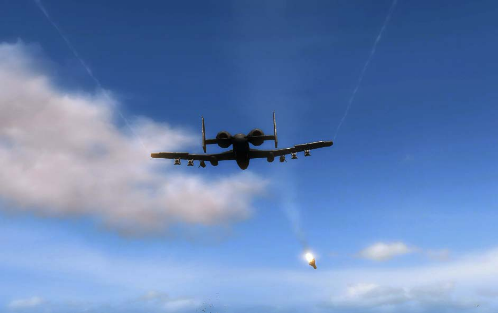
An AGM-65 Maverick missile using Electro-Optical (EO) passive seeker is seen sharply turning to align itself toward its target.
