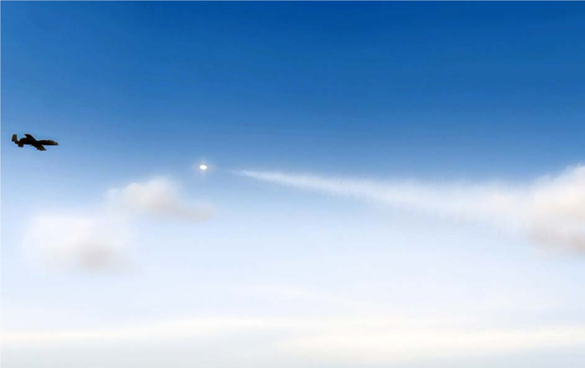
An SA-22 Greyhound (57E6-E Pantsir S1) missile is seen streaking across the sky and homing to its target using Command to Line-of-Sight (CLOS) guidance from the launch vehicle.
