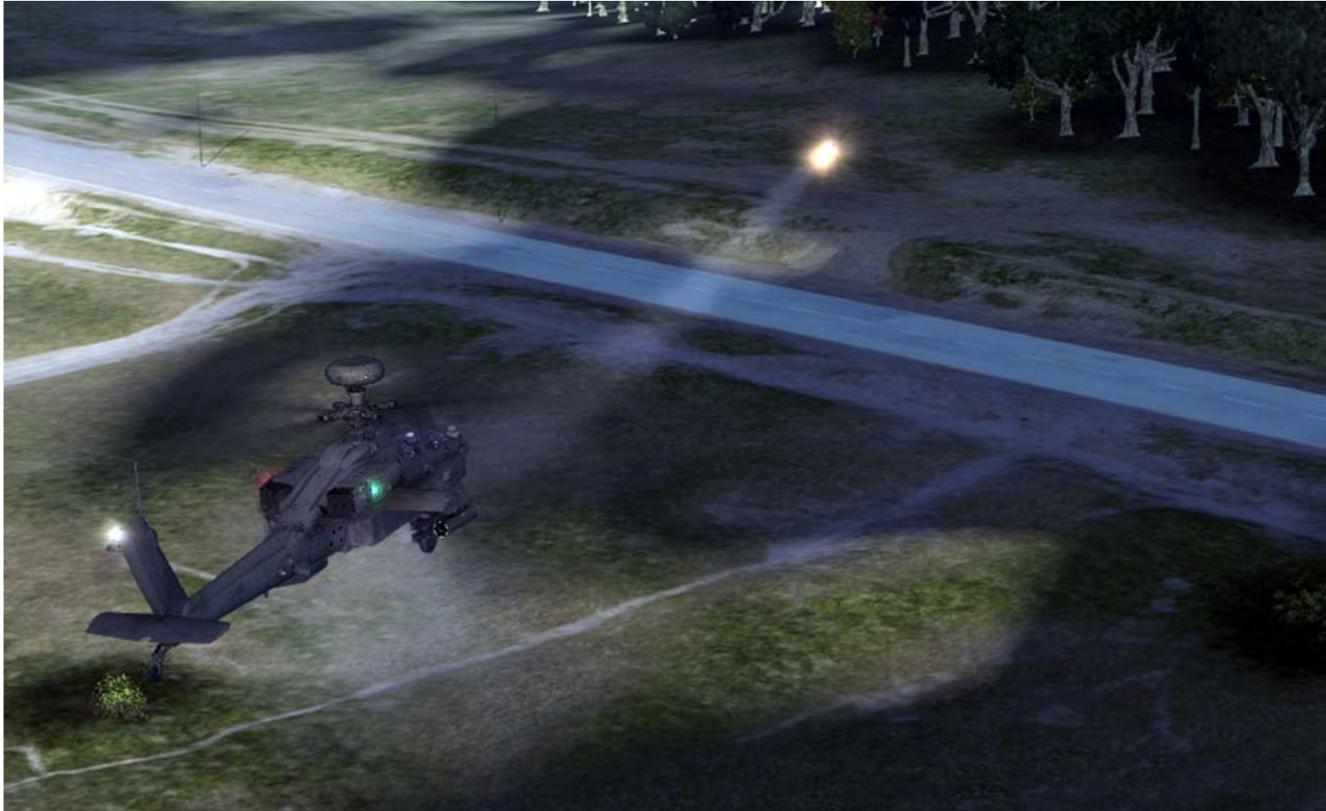
An Apache fires the AGM-114R semi-active laser homing Hellfire missile. The missile is seen pitching up and lofting into higher altitude to extend its range.
