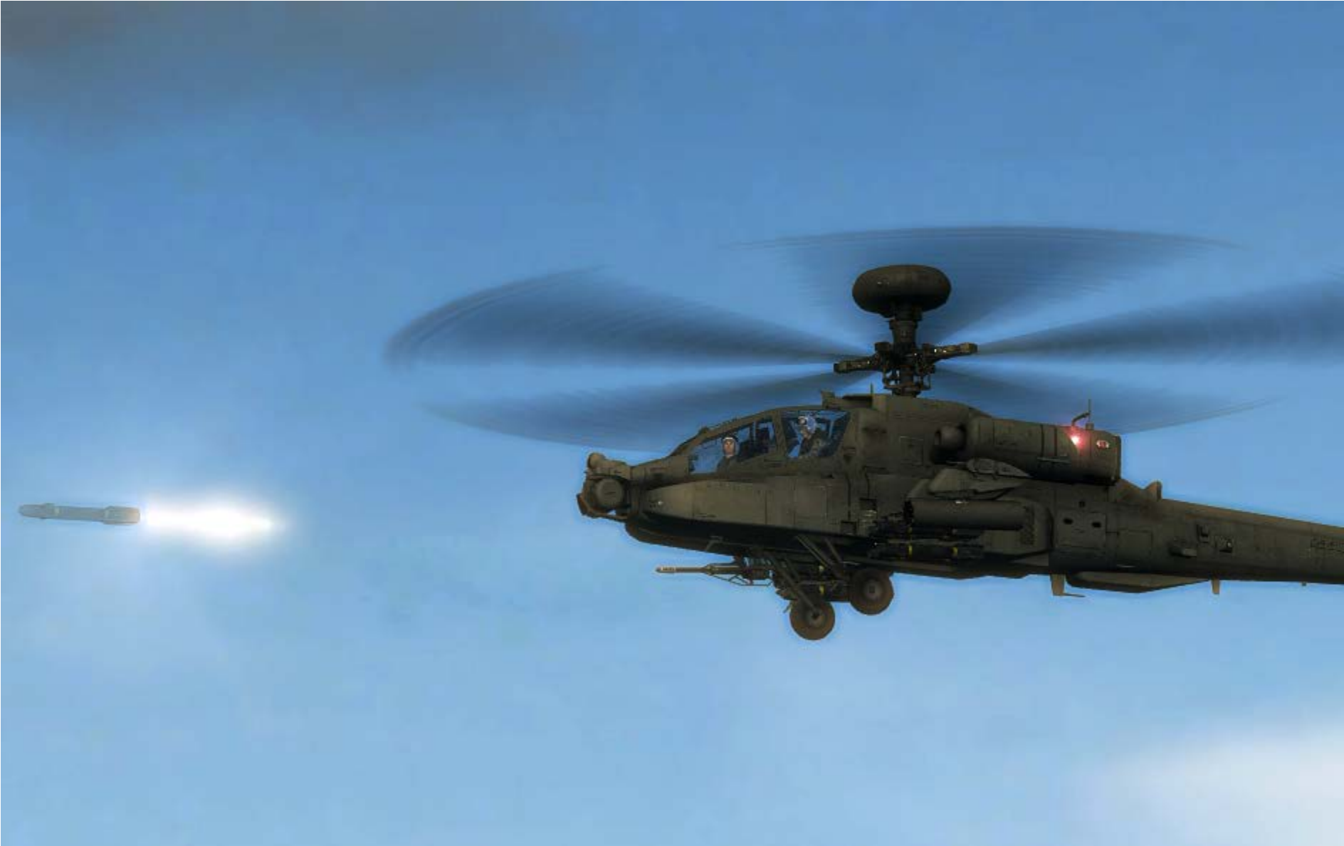
An Apache launches a Hellfire missile using Lock On After Launch (LOAL), taking advantage of the missile's inertial navigation system.
