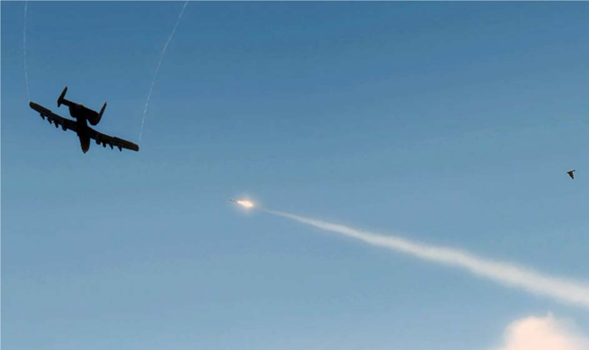
A FIM-92 Stinger missile is seen tracking an aircraft target using Augmented Proportional Navigation (APN). The missile and target appear to be on a collision course. Missile flies nearly in straight line as it approaches the target.
